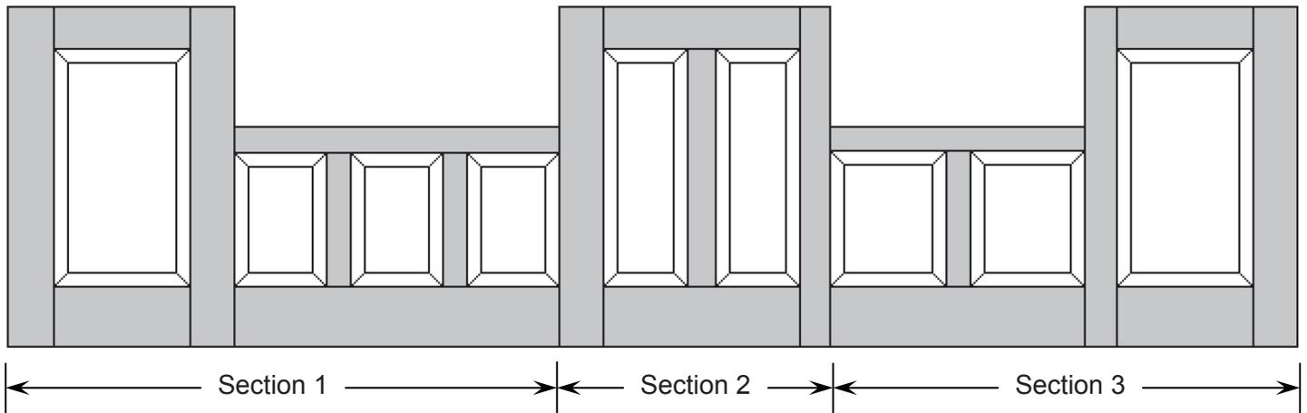
**Illustrated above is an example of how an 8' or longer wainscot panel can be split into multiple sections by extending the mid stiles - breaking the top and bottom rails.**
